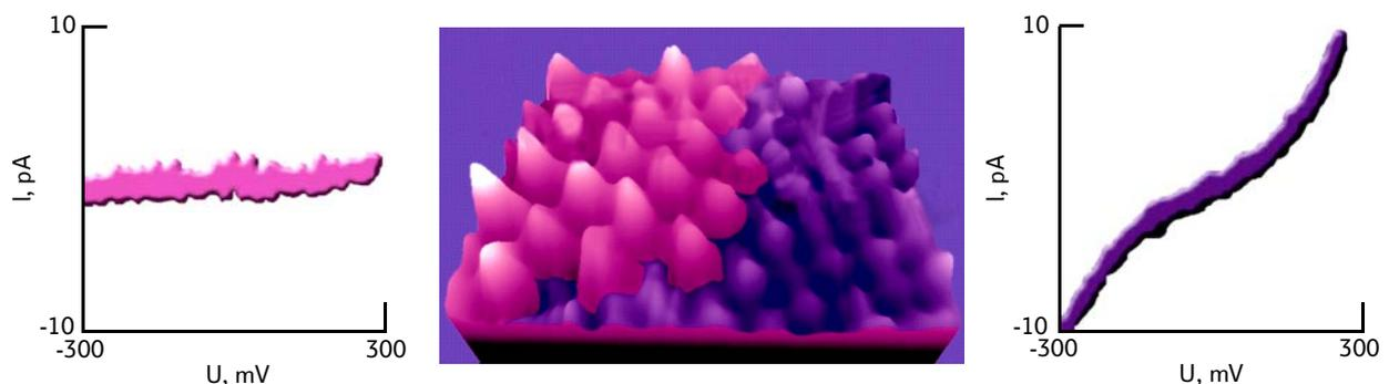
Fig 3 A stable, atomic-scale wall between regions with and without charge order (adapted from Renner et al [2]).
