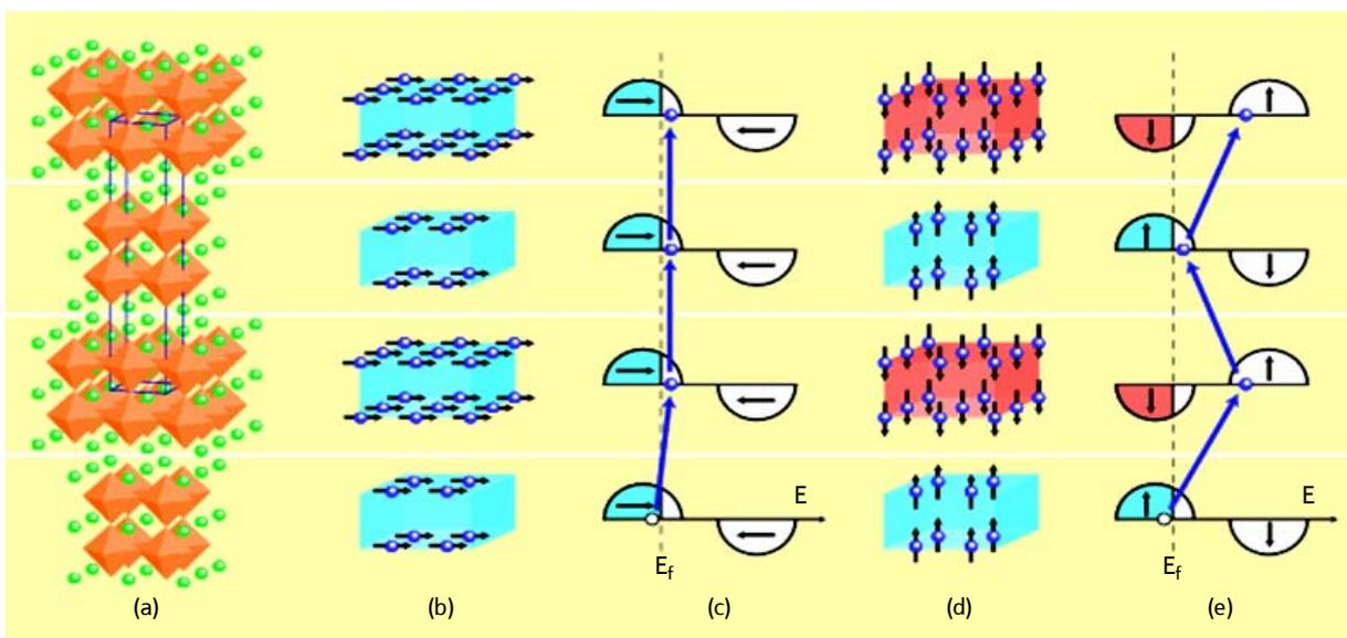
Fig 4 Self-assembled stack of tunnelling spin valves ( $\text{La}_{2-2x}\text{Sr}_{1+2x}\text{Mn}_2\text{O}_7$  with  $x = 0.3$ ) (from Perring et al [4]).
