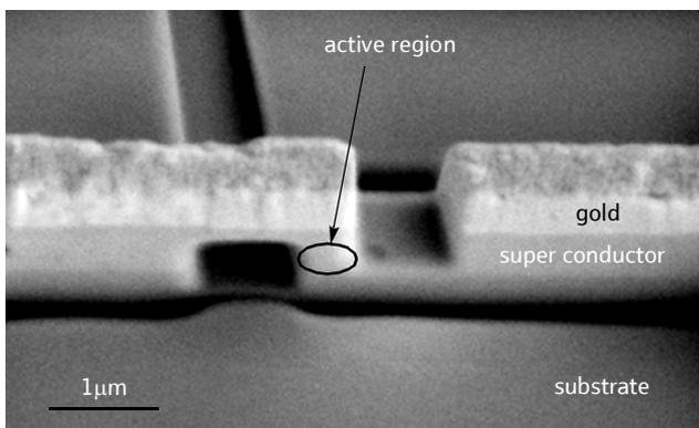
Fig 6 Self-assembled stacks of Josephson junctions in  $\text{Tl}_2\text{Ba}_2\text{CaCu}_2\text{O}_8$  [6].
