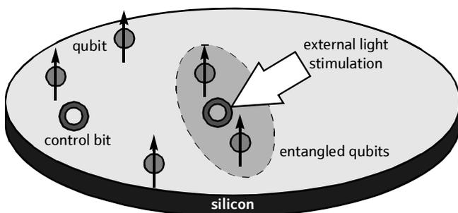
Fig 9 Schematic of a possible silicon-based implementation of a quantum computer. Spin 'qubits' are associated with the impurity atoms, and their states and quantum entanglement are controlled via optical excitation of 'control bits' associated with the electronic orbitals of the darker impurity atoms (adapted from Stoneham et al [9]).
