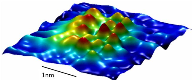
Fig 5 Trapped ‘polaron’, the texture surrounding the charge carriers in the planes of  $\text{La}_{2-2x}\text{Sr}_{1+2x}\text{Mn}_2\text{O}_7$  with  $x = 0.3$ , a ceramic layered material exhibiting two-dimensional confinement of charge carriers and therefore a prototype host for three-dimensional integrated electronics (adapted from Ronnow et al [5]).
