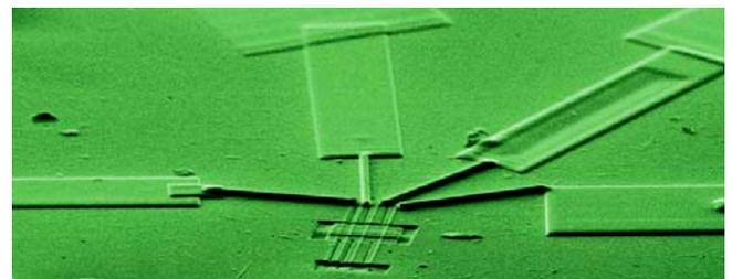
Fig 2 Four electrodes fanning out from a single isolate amyloid fibril [1].
