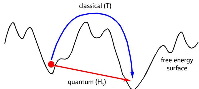
Fig 7 Schematic showing thermal and quantum annealing protocols for finding the optimum (lowest value) of an objective function, as defined — for example — for a communications routing problem (from Brooke et al [7]).
